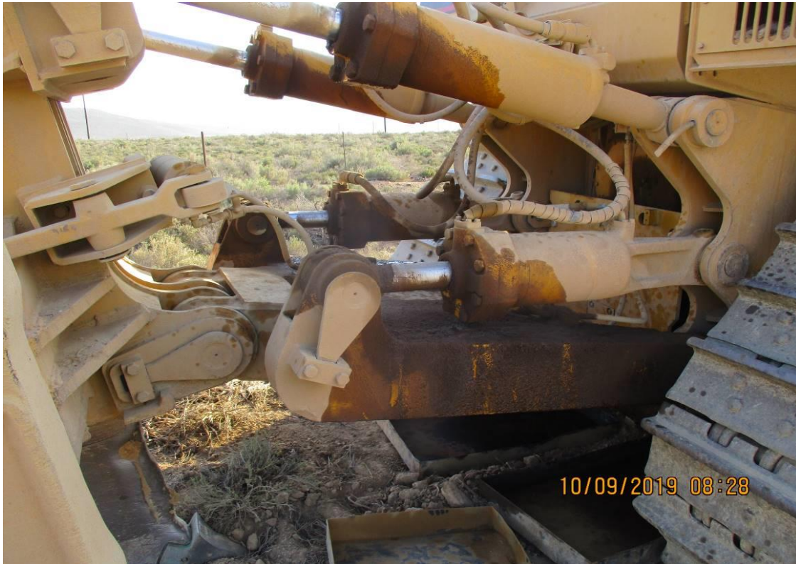
Photo: Multiple hydraulic oil leaks from the bulldozer.
