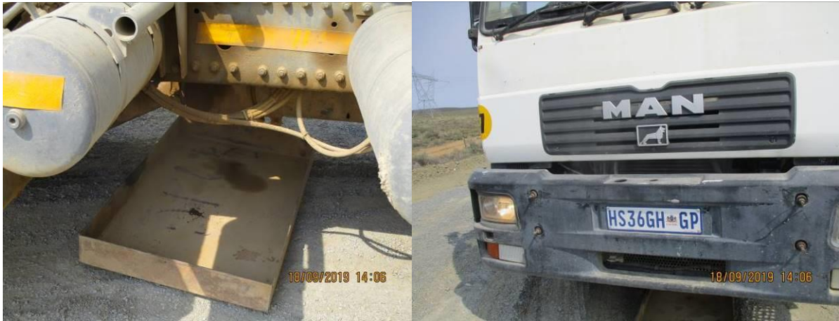
Photo: Leaking ready mix concrete truck (HS36GHGP).
