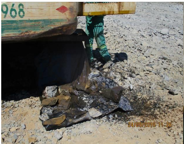
Photo: Another hydraulic oil spill from excavator (BXW 13).
